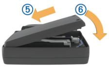
8 Close the battery cover 6 and tighten the screws. NOTE: Do not over-tighten the screws.
